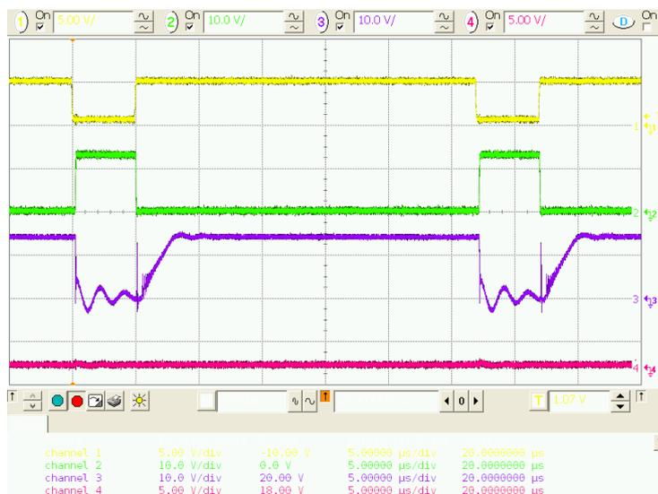
**Figure 8.12:** Oscilloscope snapshot with PWM out duty cycle = 15%
