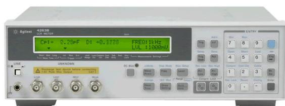
**Figure 6.5:** *Digital RLC meter Agilent 4263B*
